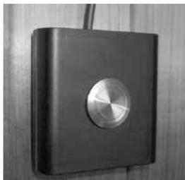
Now pull the button back off again and press the remaining adhesive tape strips down.
